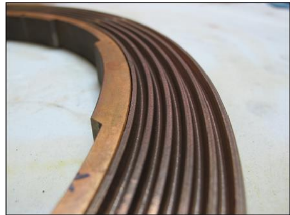
Figure 4 - Polycone clutch (side of center member)
