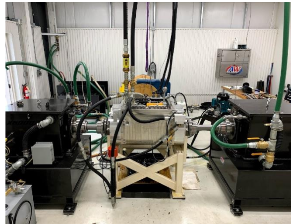
Figure 14 - ICT in test cell at KTR
